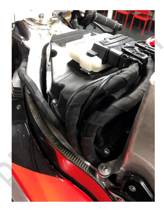
The ecu must be isolated by the engine and bike vibrations. A proper support should be adopted like as supply by Mectronik, built with a silicone enclosure and aluminum bracket. The installer should check always that none interferences between ecu assembly and other components like airbox, screws, covers and so on.
