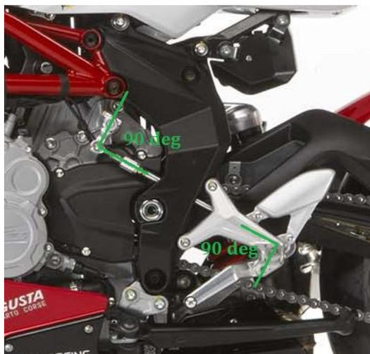
1) To have maximum torque on gearshift shaft ( internal to engine ) , with minimum rider force on leverage , the shaft where is mounted the sensor must work at 90 degree with both upper and lower leverage .
