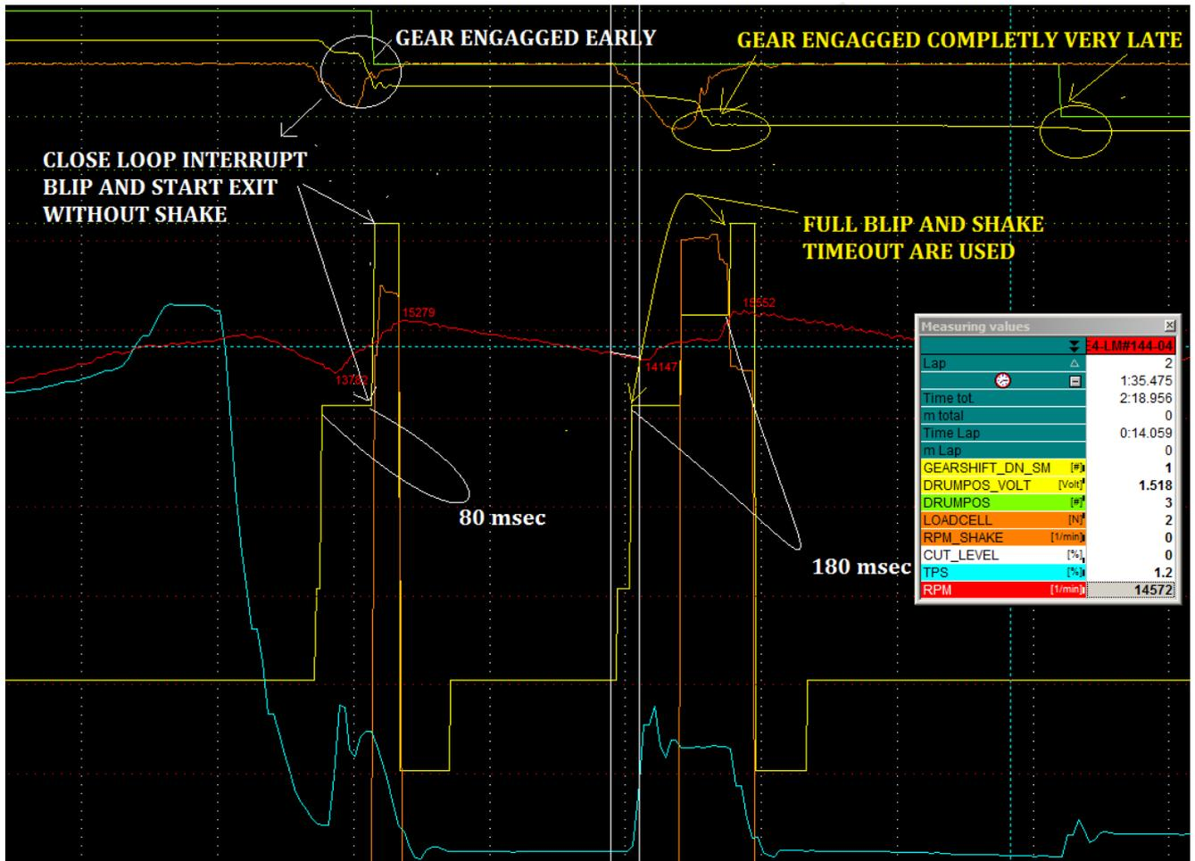
To have closed loop working fine , it's very fundamental the perfect setting of gear position sensor . Please check the related user manual for a detailed procedure .
