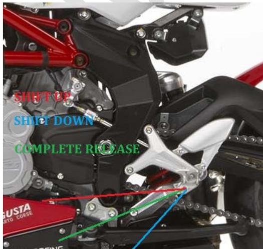
2) The leverage must be mounted for best raider comfort . It's important to remember that the leverage position at complete release , must permit to rider to release completely it after a gear shift . If it's not , the internal shift shaft , will not engage mechanism for next shifting .
