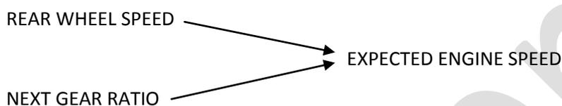
This expected ENGINE SPEED is compared with MAXIMUM RPM LIMTER , imposed by manufacturer , and in case the expected value is ABOVE the imposed limit , the trigger for BLIP is ignored .
