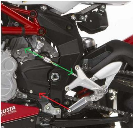
If You would like to change the leverage using a “reverse racing” version , using standard **SINGLE SWITCH** sensor , You must consider that sensor must continue to work in the same way ( extension ) . In case You have a **DOUBLE SWITCH** sensor or a **LOAD CELL** sensor , You are free to mount sensor how You like , You will configure inside the software the correct force type ( extension or compression ) for both gear shift UP and DOWN .
